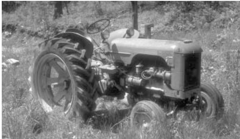
Tractors with no rollover protection structure (ROPS), such as the tractor shown above, continue to be used in the United States, despite numerous injuries and deaths resulting from rollovers.
