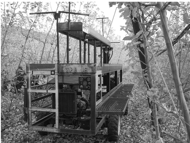
Orchard platform at Auvil Fruit Company (AFC) enables labor efficiency and safety. Note: apple trees are trained to grow in a V-shape, optimizing production and eliminating ladders during thinning, pruning and harvest.
