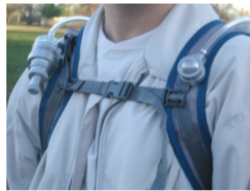
Worker wearing backpack exposure assessing system.
