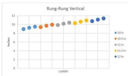
The vertical distance between rungs is dependent on both the rung spacing and the ladder angle. This chart shows these distances for each ladder at each angle. There is a general progression upwards, with a slight dip in distance between the one ladder at its steepest angle to the next larger-spaced ladder at its shallowest angle.
