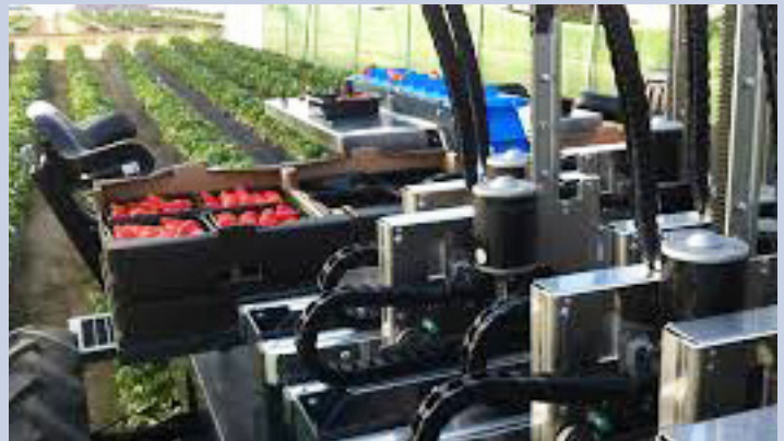
Agrobot strawberry harvester picks ripe strawberries for packing
