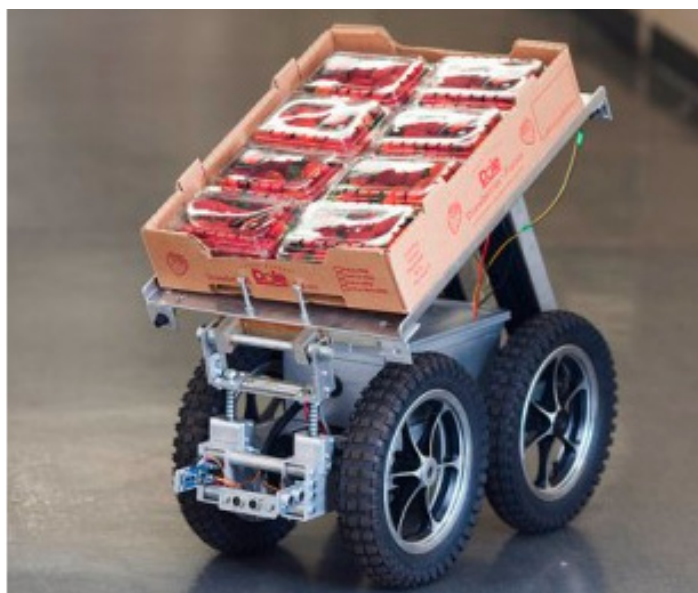
The co-bot is designed to fit within the strawberry field furrows by being small and sturdy, with heavy-duty wheels.
