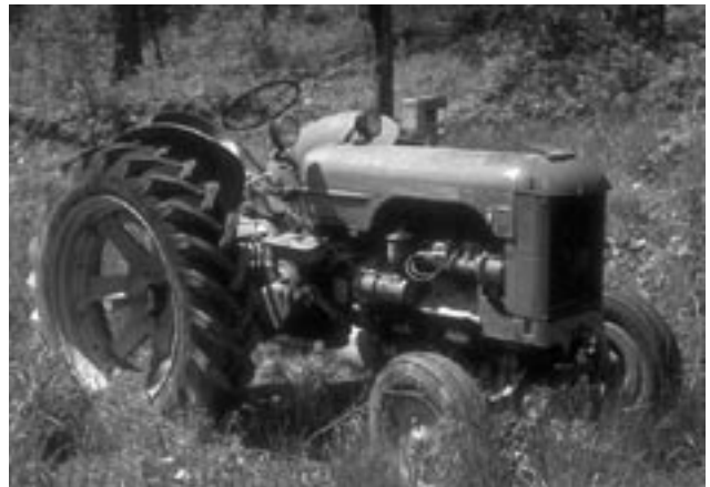
Old tractor with no rollover protection (ROP)
