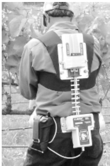
The lumbar motion monitor (LMM), shown above on a vineyard worker, mimics the spinal column, while registering the motion of a person engaged in different work situations.
